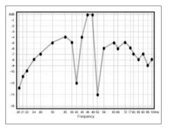
Figure 19. Example of two narrow dips
