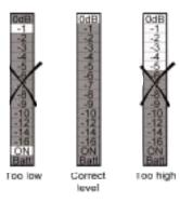
Figure 5. Adjusting the subwoofer levels for a 0dB peak When finished, press Pause II.
